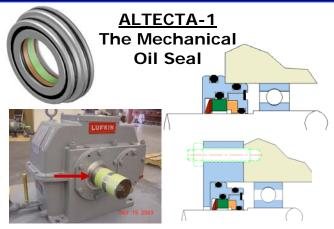
ALTECTA-1 is a "cartridge mechanical oil seal" which built durable than any other Bearing Seals in the market such as; Lip Seal, Labyrinth & Magnetic types seal. ALTECTA-1 designed to function in low speed or high speed and wet or dry application. It performs in atmospheric, mist lubrication, film lubrication, high oil level or oil flooded conditions.
