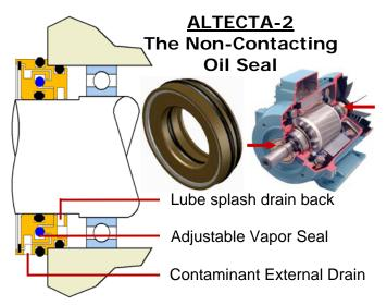
ALTECTA-2 is a "non-contacting oil seal", designed for electric motors, pumps and other high speed rotating equipment not below 350 rpm. ALTECTA-2 has adjustable vapor seal that automatically lift when shaft rotates and return to contact with stator and rotor when shaft stop.
